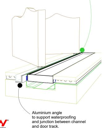
For all types of threshold installation ensure both sides of the channel are sealed before laying tile.
