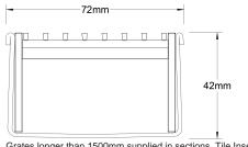
Grates longer than 1500mm supplied in sections. Tile Inserts longer than 1200mm supplied in sections. Channels over 3000mm supplied in sections with joiner. +/-2mm tolerance on
